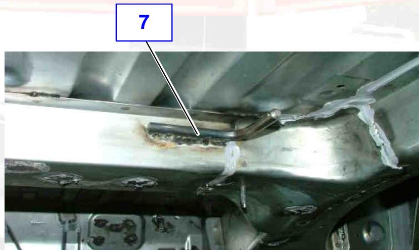
B - Welding the mount wire on the rear moulding (ref. 7).
