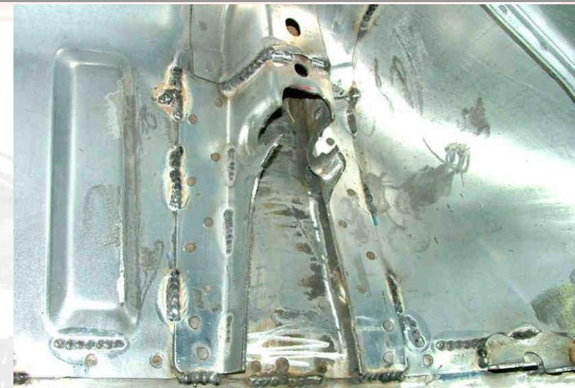
Flatten the plate in the area shown (shock absorber upper housing passage)
