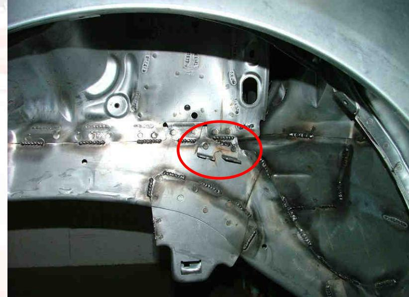
Carefully unstick the right and left front flexible hose mount, using a removing bit. The mount must not be damaged during this operation.
